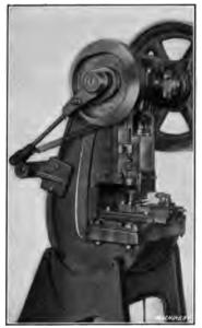
Fig. 7. Press Equipped with Slide Feed Mechanism
